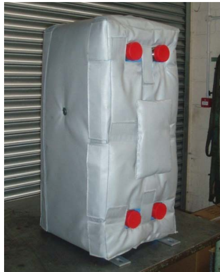
Fig.2 Insulation GL-13 Heat Exchanger
