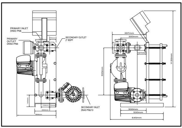
Recommended Minimum Clearances: 450mm front, 300mm primary pump side, 150mm other side
